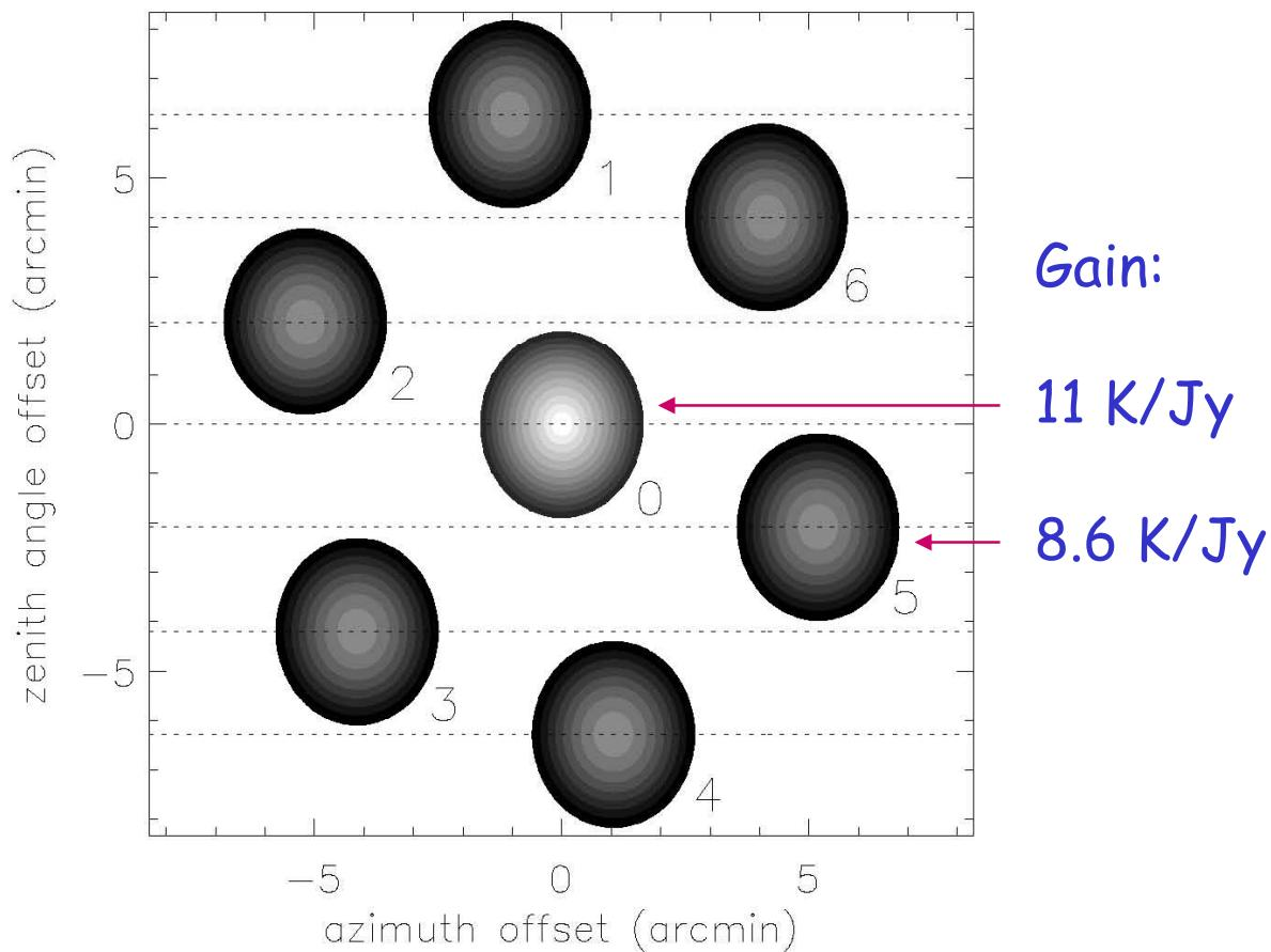
Fig. 2.— Sketch of the geometry of the ALFA footprint, with the array located along the local meridian and rotated by an angle of  $19^\circ$  about its axis. The outer boundary of each beam corresponds to the  $-3$  dB level. The dashed horizontal lines represent the tracks at constant Declination of the seven ALFA beams, as data is acquired in drift mode.
